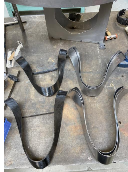
3D printed guide to ensure the steel arcs match.
