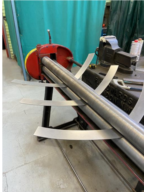
Used the roller, rubber mallet, and anvil to hand-bend the laser cut steel.
