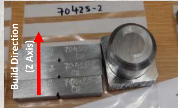
a) V-notch geometry
