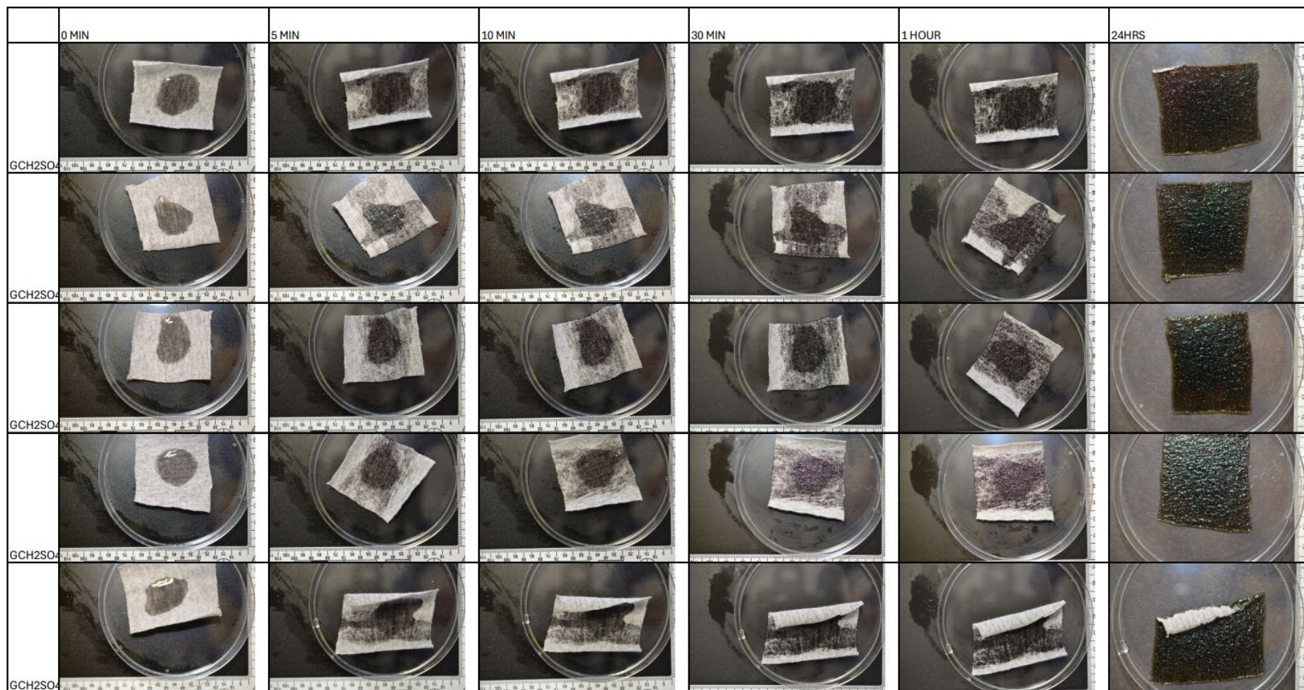
Figure 42: Sulphuric Acid - 40% on Grey Cotton
