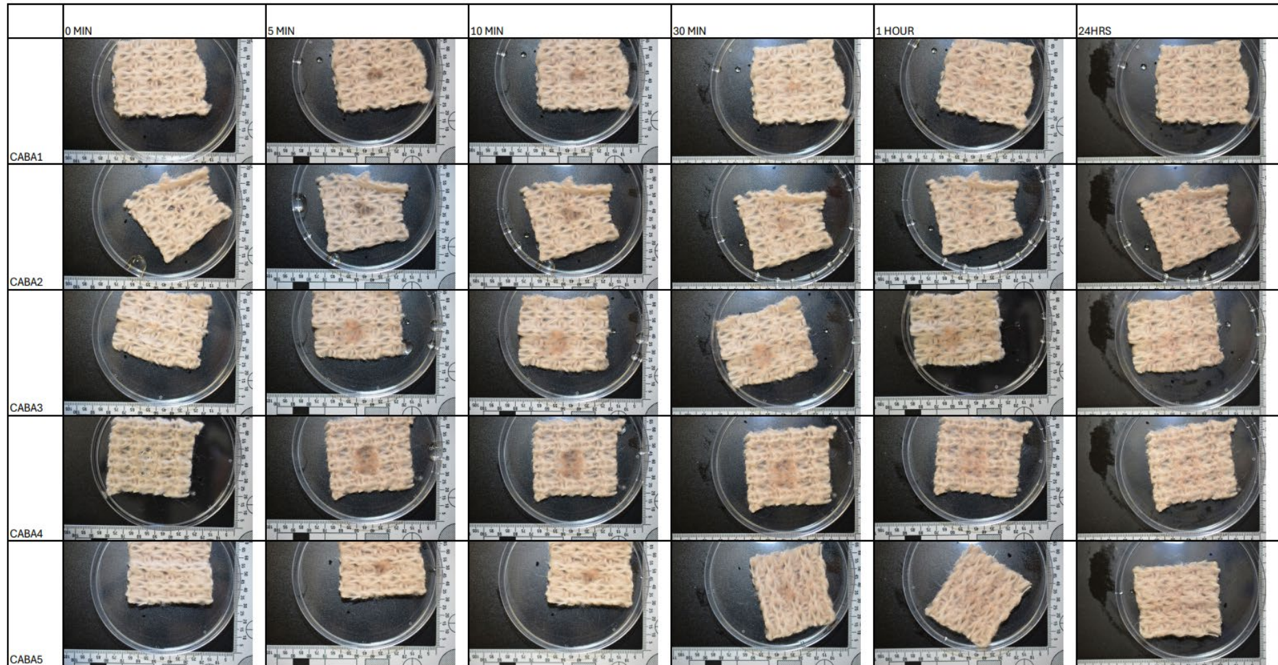
Figure 45: Sulphuric Acid - 40% on Cream Acrylic
