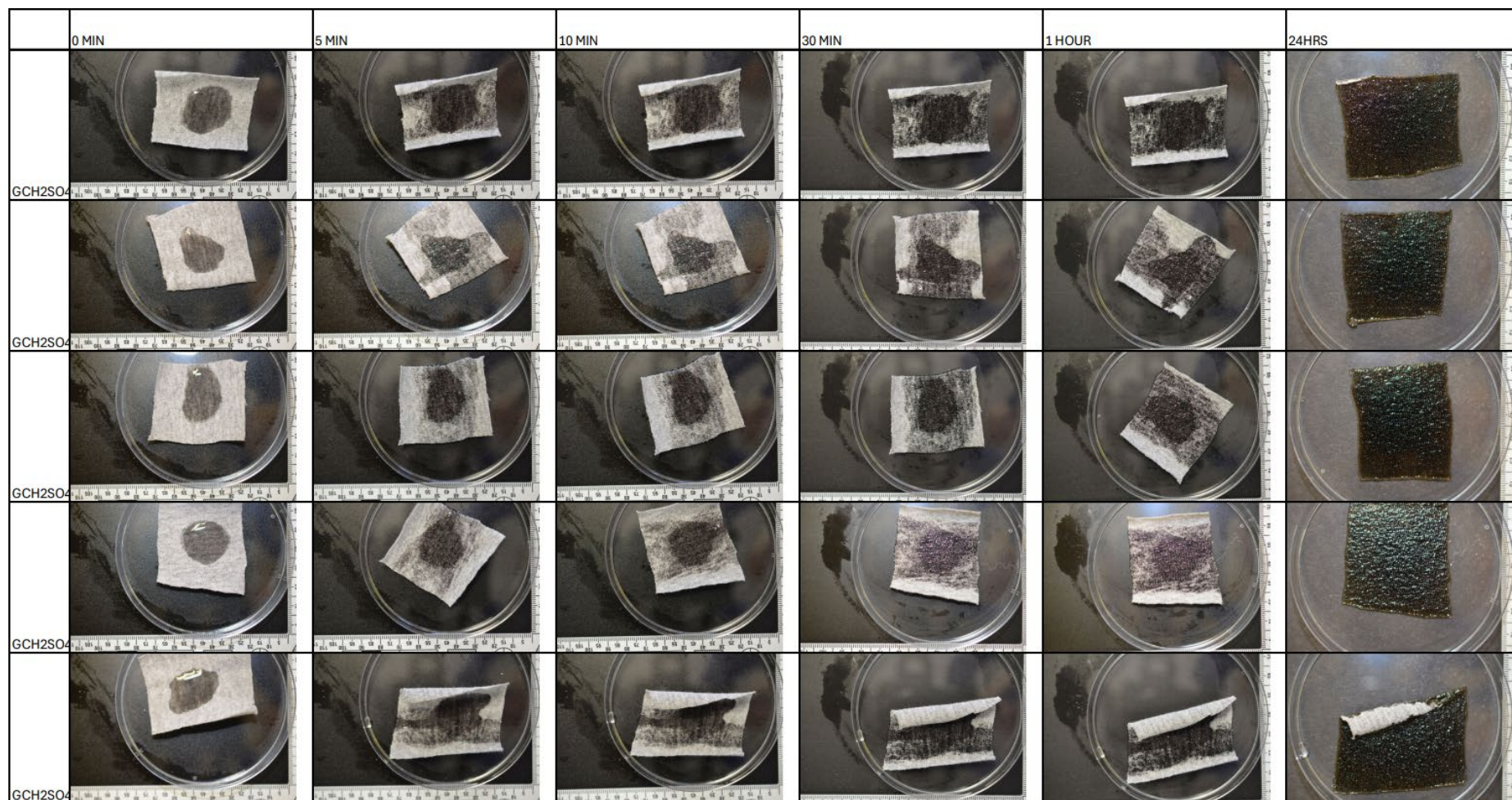
Figure 22: Sulphuric Acid - 80% on Grey Cotton
