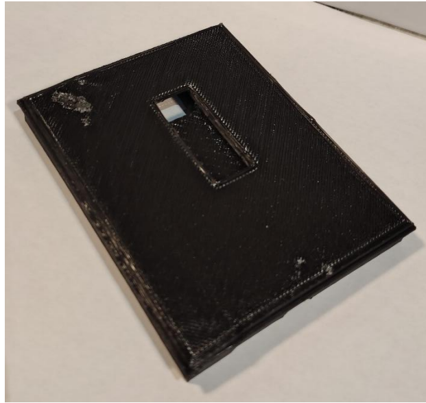
Figure 3-25: Misprint of the Mk.4 lid due to the support material failing to disconnect properly
