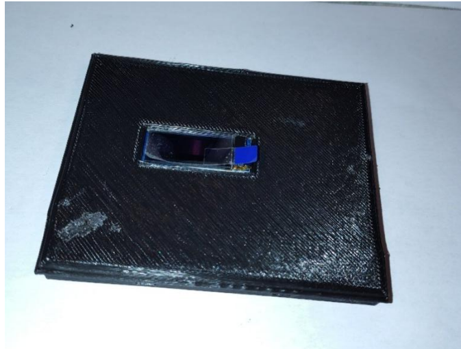
Figure 5-7: Mk.4 Lid with OLED screen in place (Top)
