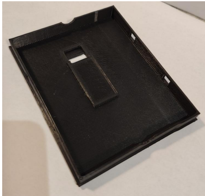
Figure 3-26: The underside of the misprinted Mk.4 lid, showing no defects
