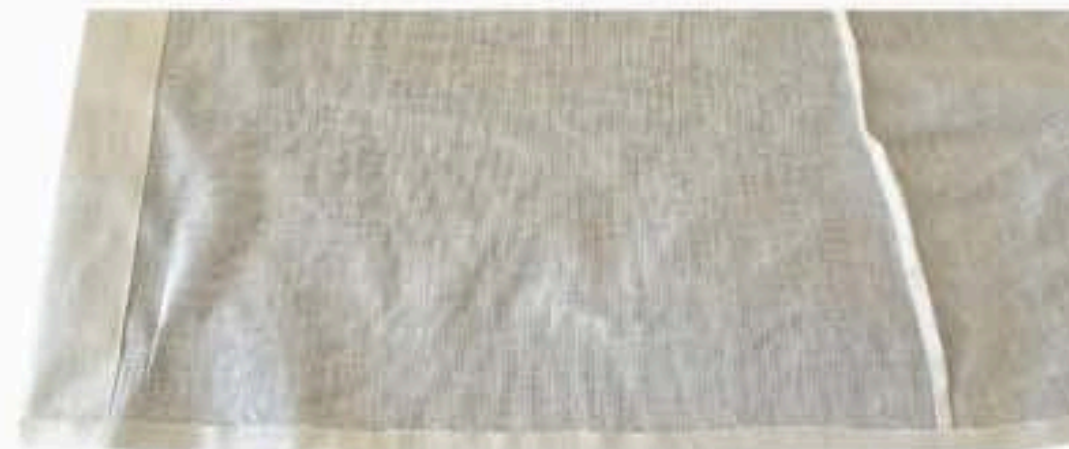
Shirt Hem Finished with 1cm Double Turn Hem; Topstitched 1mm from Edge for a Clean Finish
