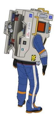
Place internal straps over shoulders. Assistance will be required to lift the suit.
