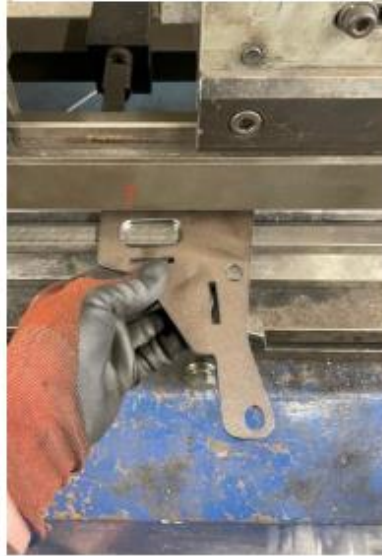
Bending (press-braking) the sheet metal brackets.
