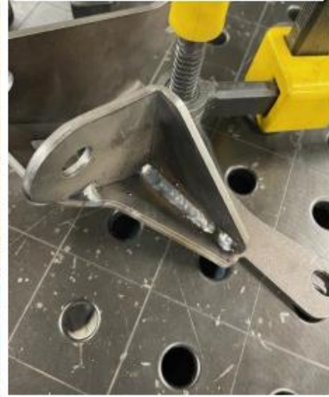
Welding the two brackets together to make the steering arm.
