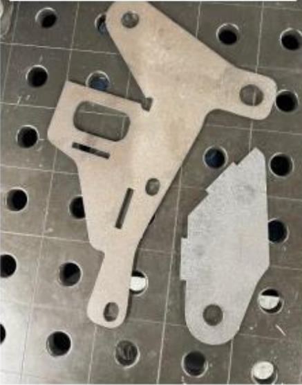
The laser-cut flat 4mm sheet metal steering arm components.
